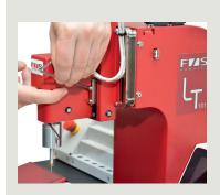
Exchangeable test-cartridge for thin- and heavy wire
